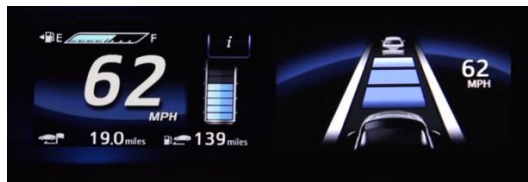
Examples of FCEV display panels showing SOC and estimated range
