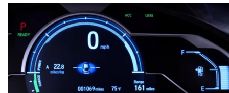
Examples of FCEV display panels showing SOC and estimated range
