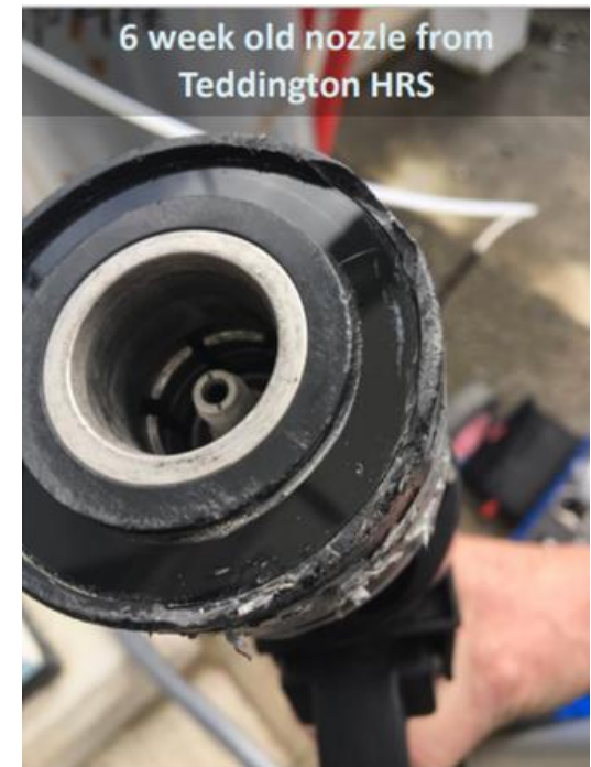
Picture of a HRS dispenser nozzle damaged by users (Credit: ITM Power)
