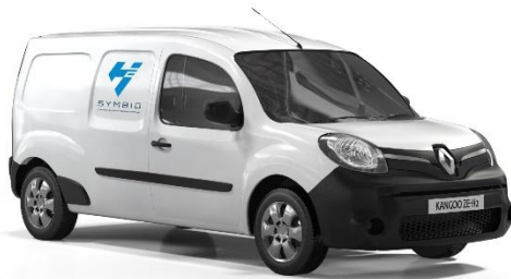
Renault van equipped with Symbio FC range extension system, France
